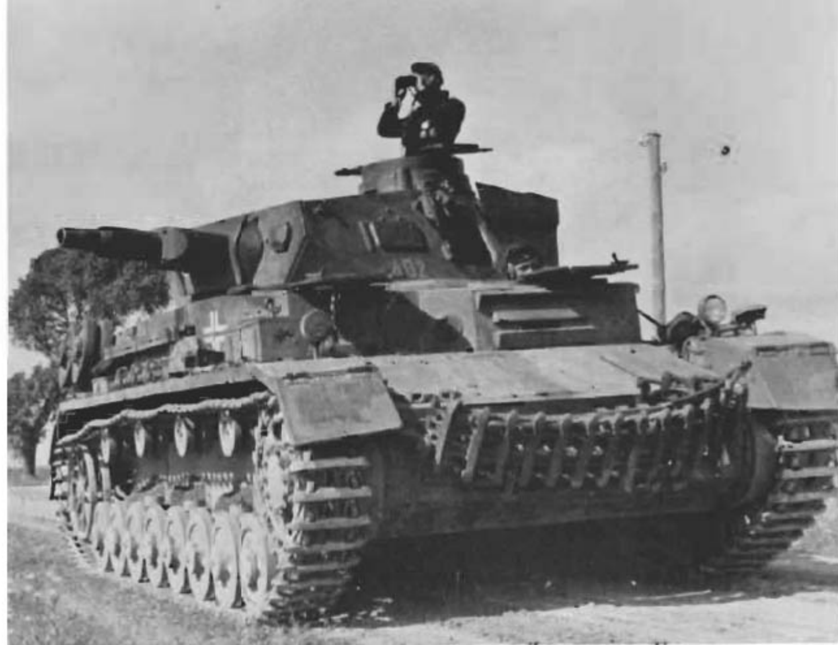
PzKpfw IV ausf D during "Barbarossa", serving with 6th Panzer Division. Again note somewhat later fittings typical of 1941 - spare track in front, and the turret stowage box. Note the rain shield over the driver's visor. The set-back R.O.'s front plate and connecting plate are seen by the way they catch the light. (Bundesarchiv)
