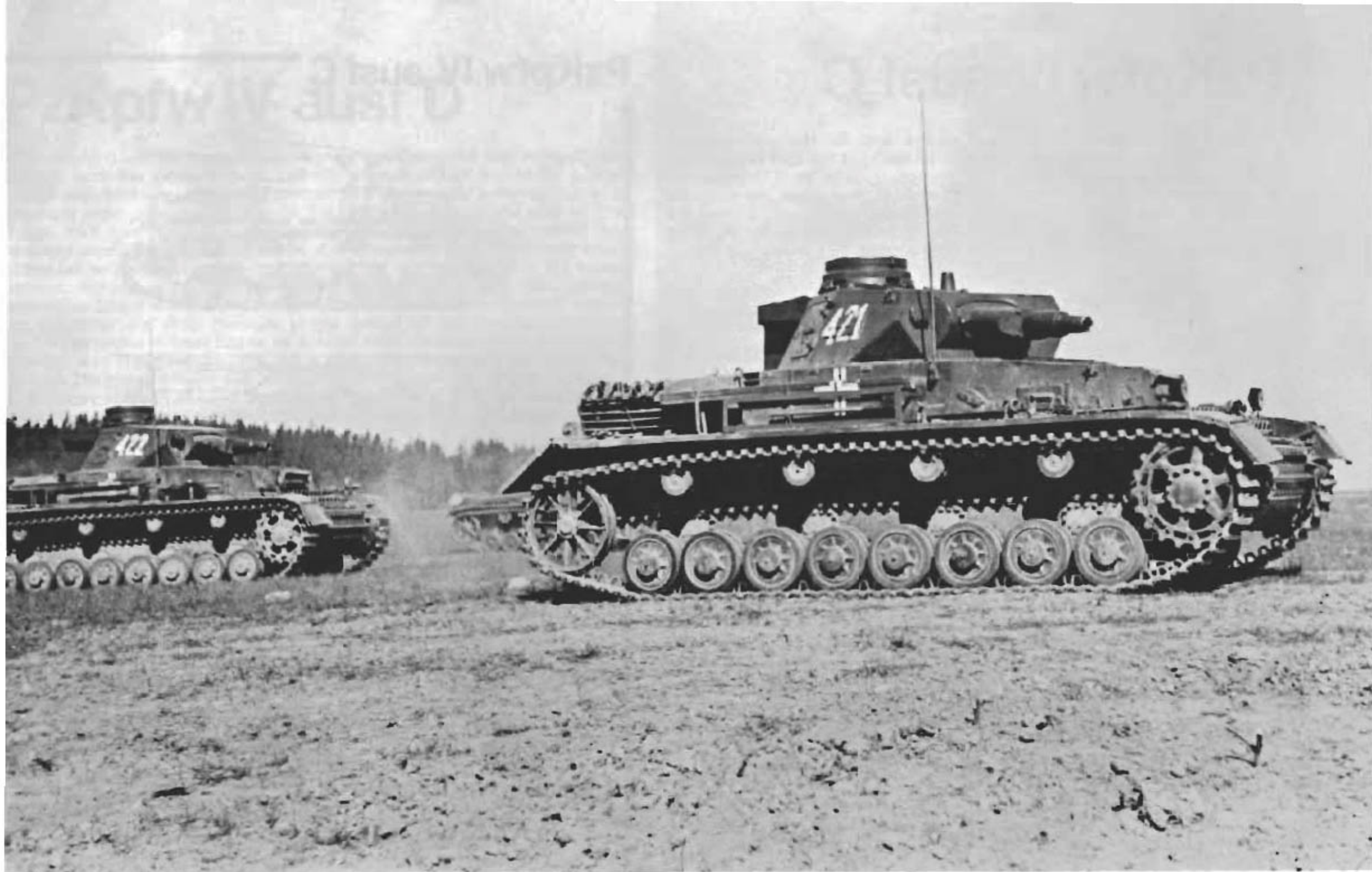
Ausf B's during "Barbarossa", the invasion of Russia. The basic appearance of this early PzKpfw IV is very similar to all the subsequent versions. Though not too clear in this photo, the ausf B had a straight front plate. The conical structure to the right of the cupola is a covered signal port, used to shield signal lamps - a front slit allowed a narrow light beam forward. These vehicles have been retrofitted with turret stowage boxes. (Bundesarchiv)
