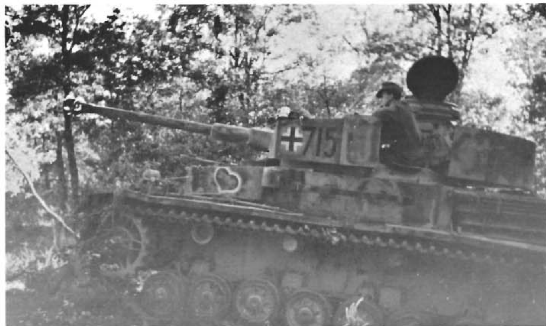
An ausf H, not fitted with hull skirting or brackets. The crew has sprayed white in a vertical wave pattern over the turret skirts. The chassis was not usually repainted. (Bundesarchiv)
