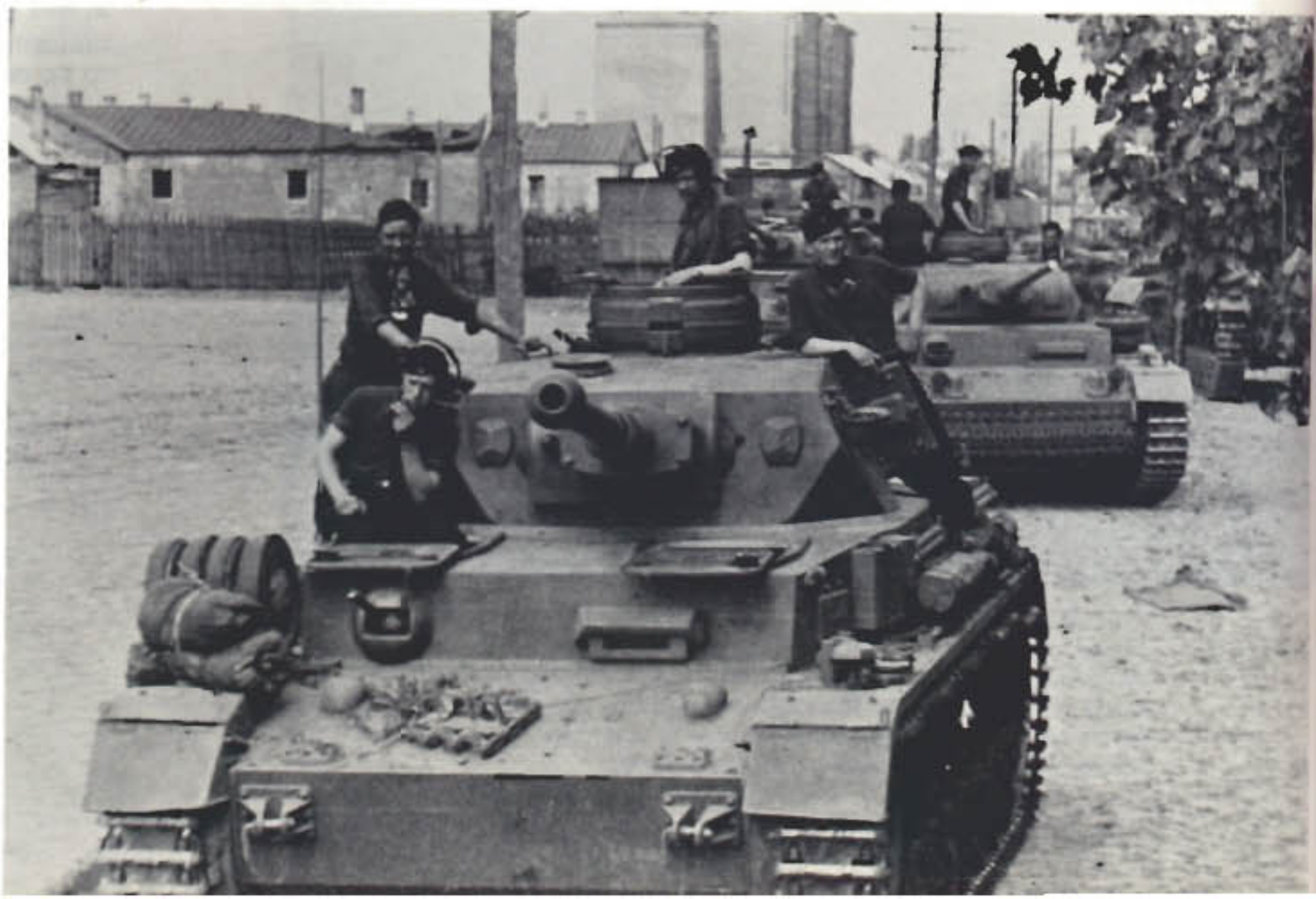
The Afrika Korps used a number of ausf F2's, though the short barreled earlier versions were much more numerous. The British often called the F2's "Mk IV Specials". The vehicle here is painted in overall "sand-brown", the second tropical sand color used by the DAK. Other than the crosses on the superstructure sides, there are no other markings on this vehicle. The globular single baffle muzzle brake used on the F2 shows well here. (Bundesarchiv)
