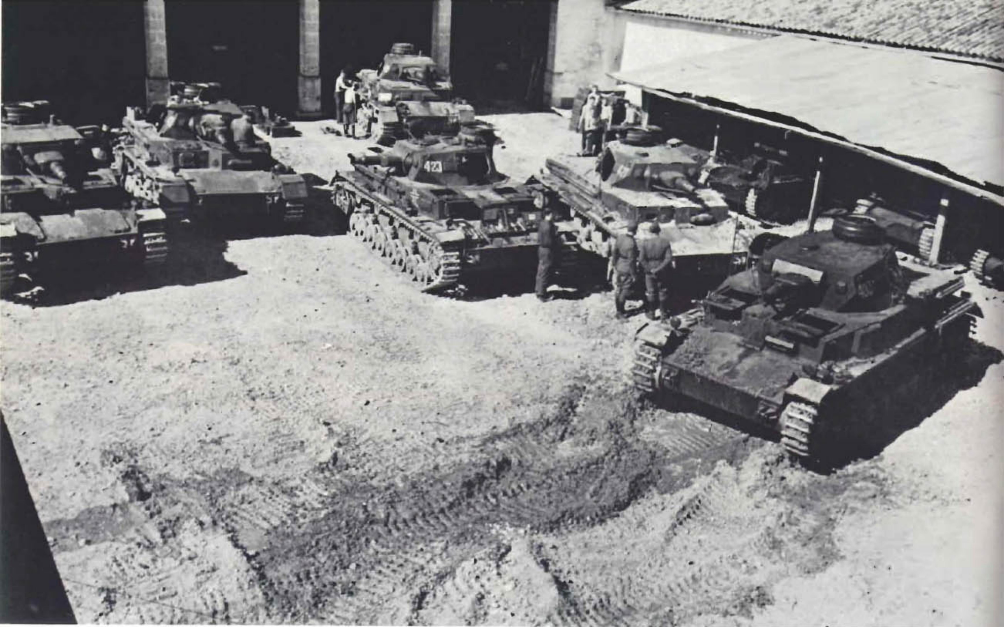
A group of ausf D and E vehicles in France after the campaign of 1940, showing the detail differences between the two models. The tanks on the far left and third from left are ausf D's; second from left, second from right, and near right are ausf E's. The vehicle second from the left is fairly unusual
