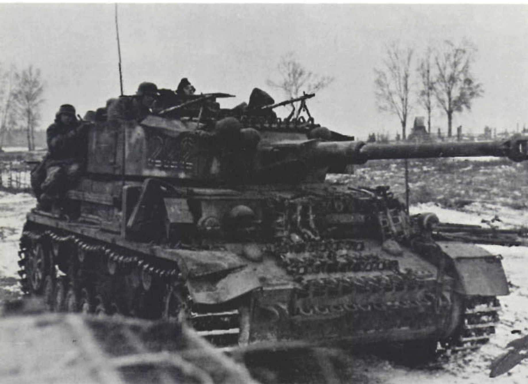
This late production ausf G in Russia, 1943, is primarily dark yellow with a desultory overspray of white stripes and spots, and white stencilled turret numbers. Note the folding radio antenna and trough and the G pattern drive sprocket. (Bundesarchiv)
