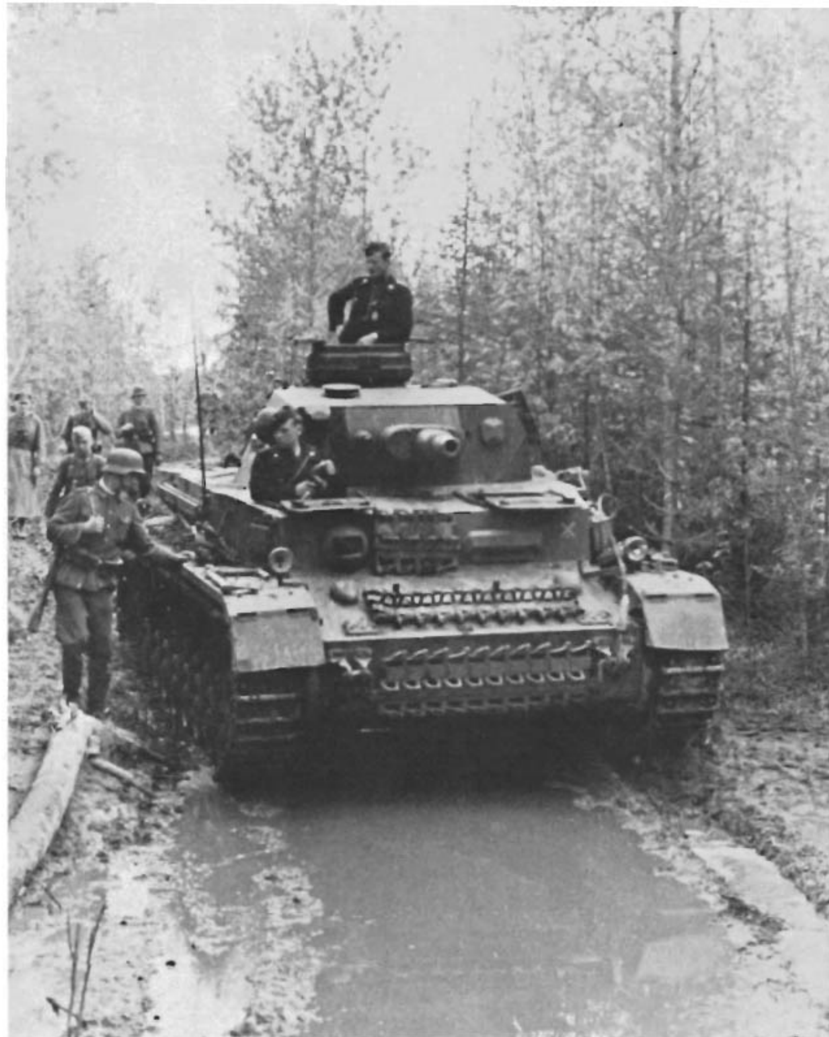
An ausf F from the 5th Panzer Division in Russia, 1941. The right side headlight is broken - this seems to have been common, and may have been caused by muzzle blast from the main armament. Even on this fairly new vehicle without apparent combat damage, the mudguards are already slightly damaged. Note the straight front plate, similar to that of the ausf B and C. (Bundesarchiv)
