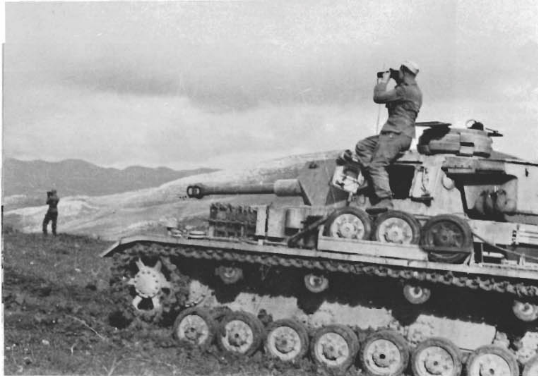
An ausf G during the winter of 1942-43. This vehicle has been repainted in overall dark yellow base color - note that the inner surfaces of the side doors are in the earlier dark gray, the original base color. Note the details of the cleaning rods. (Bundesarchiv)
