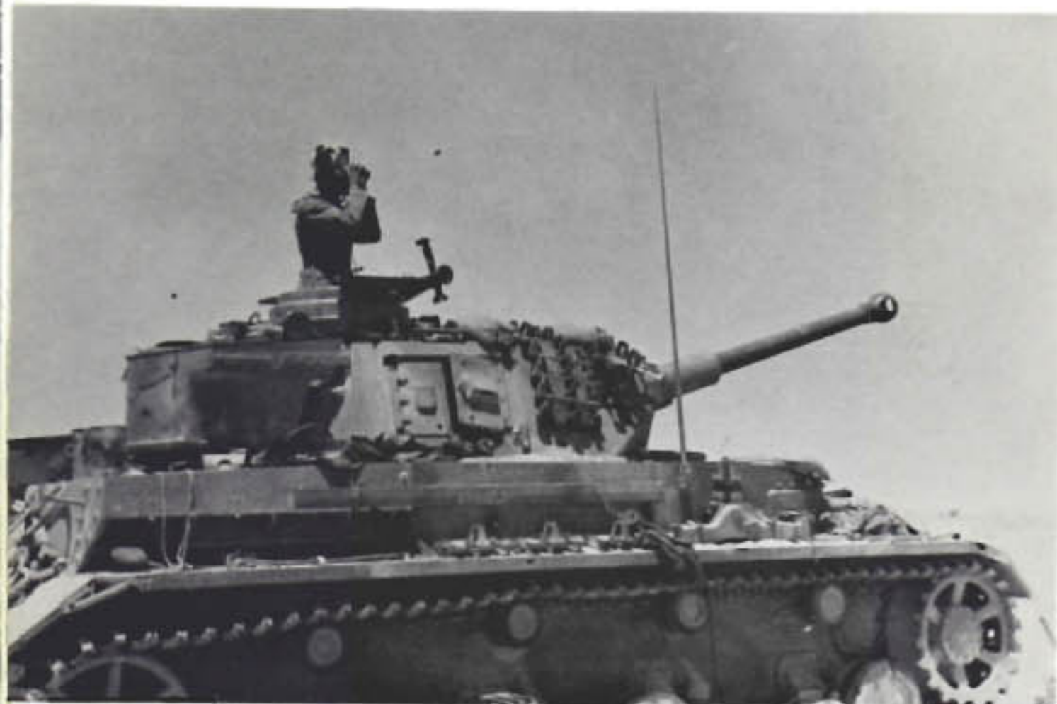
The Afrika Korps used a number of ausf F2's, though the short barreled earlier versions were much more numerous. The British often called the F2's "Mk IV Specials". The vehicle here is painted in overall "sand-brown", the second tropical sand color used by the DAK. Other than the crosses on the superstructure sides, there are no other markings on this vehicle. The globular single baffle muzzle brake used on the F2 shows well here. (Bundesarchiv)
