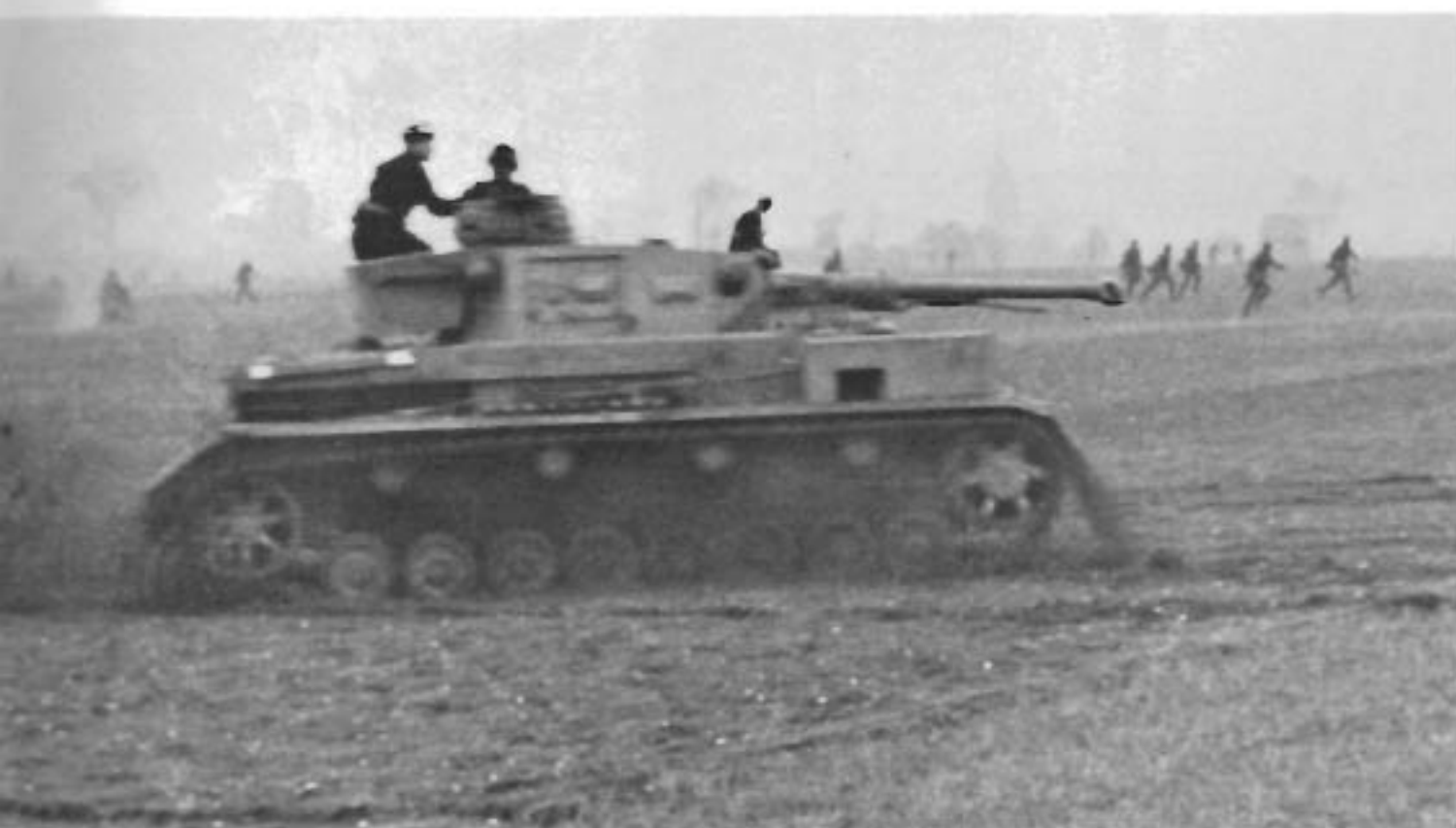
This ausf F2 was photographed during training in France, 1942. Many Panzer Divisions were badly mauled in the Russian campaign and were sent back to France for rest and refitting. The large stowage box on the right mudguard was fitted to some F2's, and a similar box was used on some ausf G's, but they were not fitted to all these models. (Bundesarchiv)
