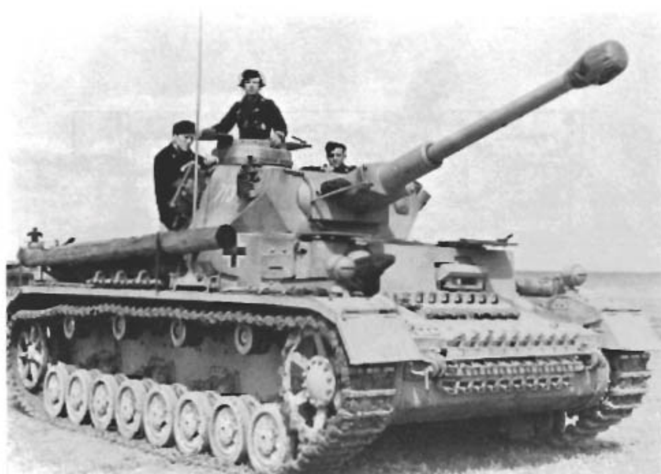
This PzKpfw IV ausf G shows the added 30mm nose and front armor as well as smoke grenade tubes, headlamps, stowage, and the standard ausf F-G suspension. This vehicle again is overall dark yellow. (Bundesarchiv)
