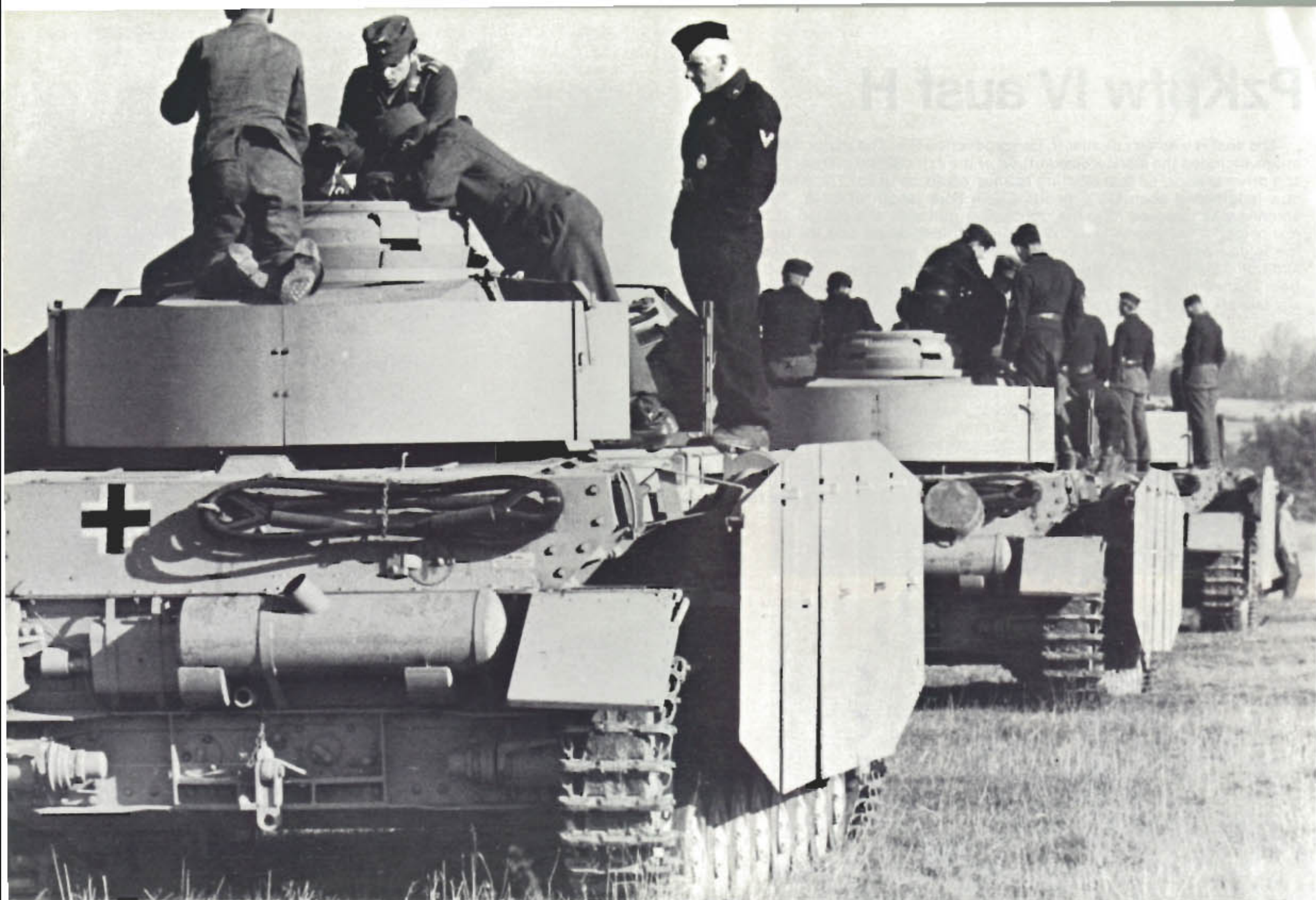
These new ausf H's in Russia show an early skirt and bracket arrangement, almost identical to that used for the PzKpfw III. In this design the skirt sections were hung on hooks from the side rails, and had cutouts for these
