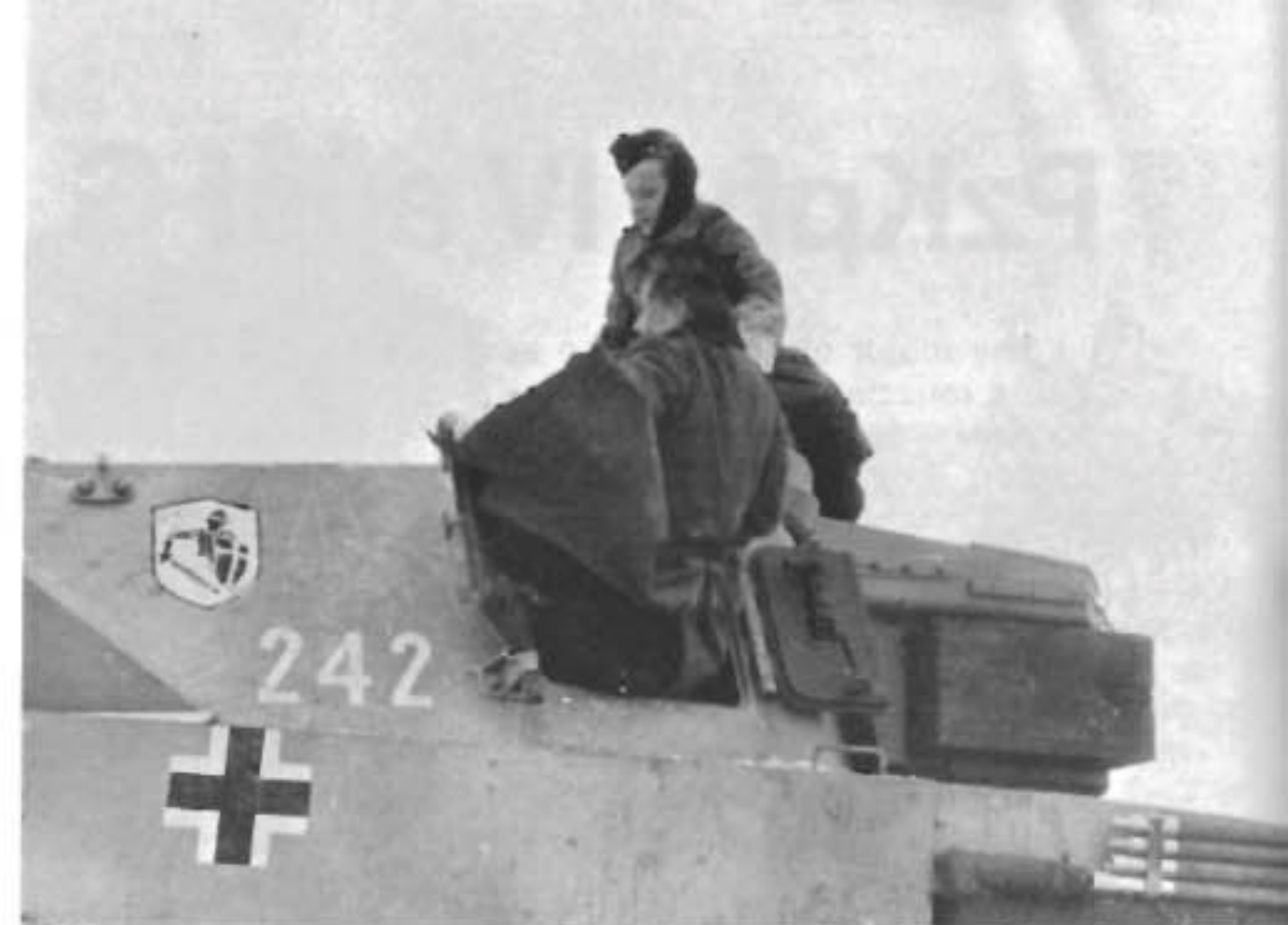
An ausf G during the winter of 1942-43. This vehicle has been repainted in overall dark yellow base color - note that the inner surfaces of the side doors are in the earlier dark gray, the original base color. Note the details of the cleaning rods. (Bundesarchiv)
