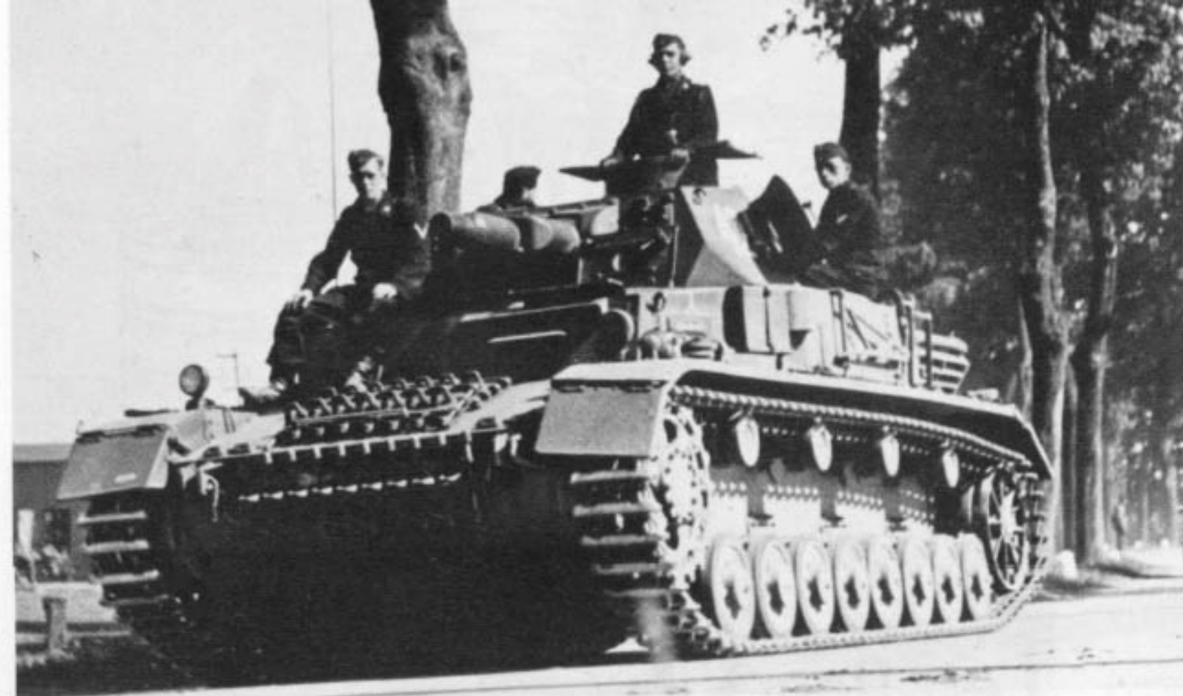
A rare view of the PzKpfw IV ausf A in action, this photograph shows a vehicle of the 1st Panzer Division in 1941, probably in France where several Panzer Divisions refitted after the campaign of 1940. The black panzer uniforms are worn with the early field cap rather than the beret. Note the early cylindrical cupola, and the added tracks used for extra protection.
